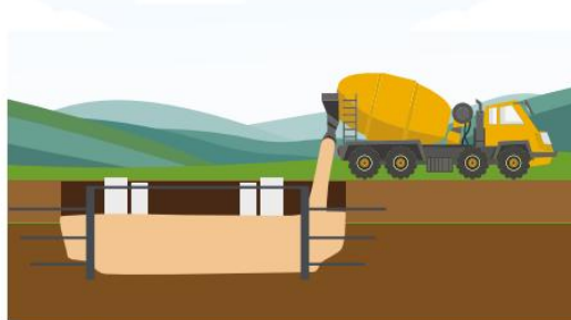
Stage 2: Pylon foundations
